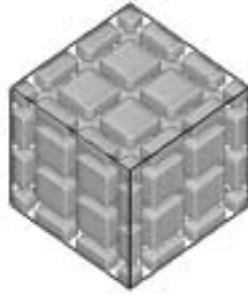
Figure 3.4: Model Structure used for the simulation of crystalline polymer (The only crystal part is shown).
